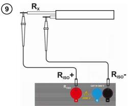
Connect test leads according to the drawing.
