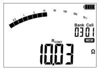
Set the bank number to be deleted acc. to section 4.2. Set the **cell number** as "--" (before "01")...
