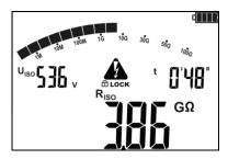
View of the screen during measurement. LOCK means that the measurement was started with ENTER button or by pressing and holding START button for approx. 5 sec.
